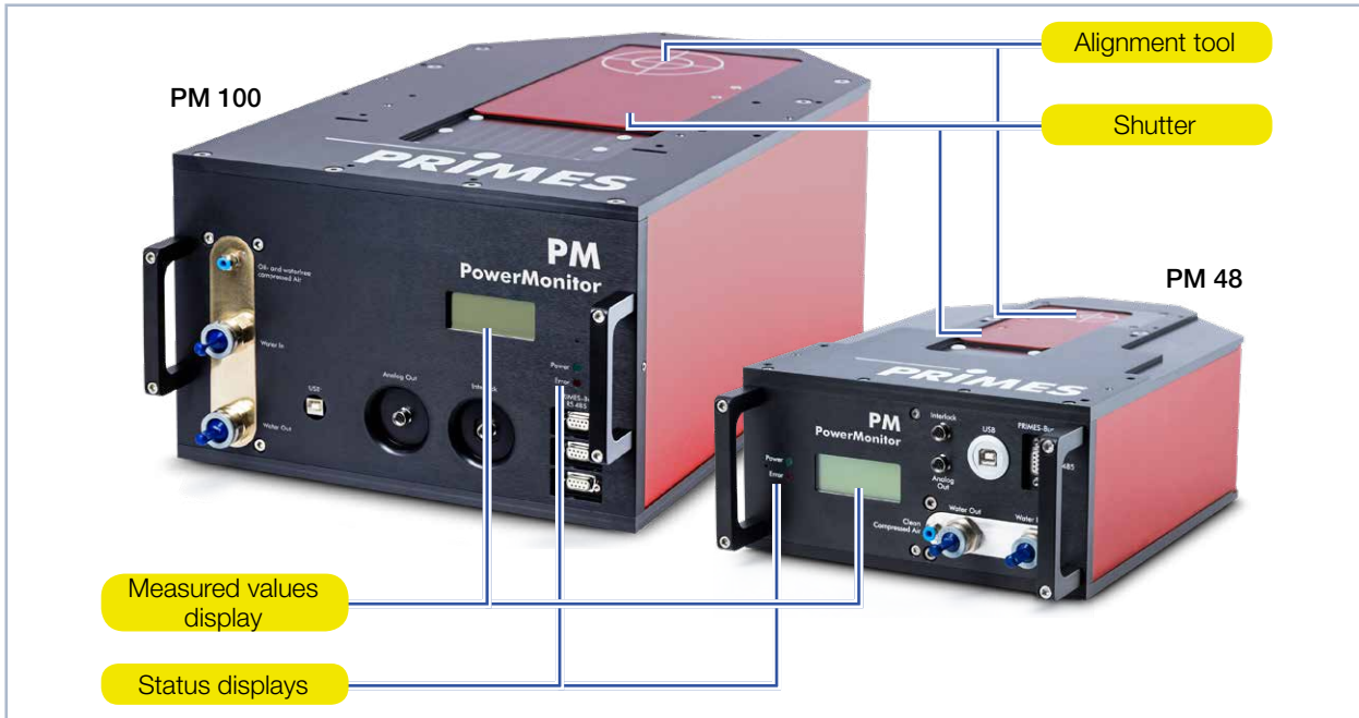
Fig. 5.1: Components of the PowerMonitor PM
